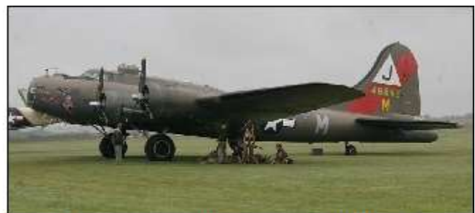
A B-17 weighs over 18 tons empty and has a wing span of 103 feet. Photo from delpinmedia
